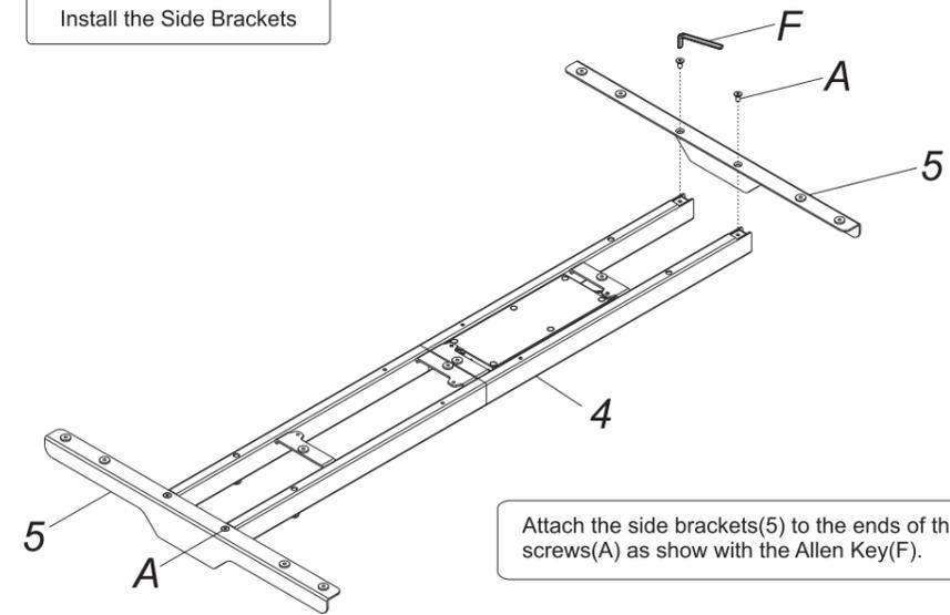
Attach the side brackets(5) to the ends of the supporting beam (4) using screws(A) as show with the Allen Key(F).
