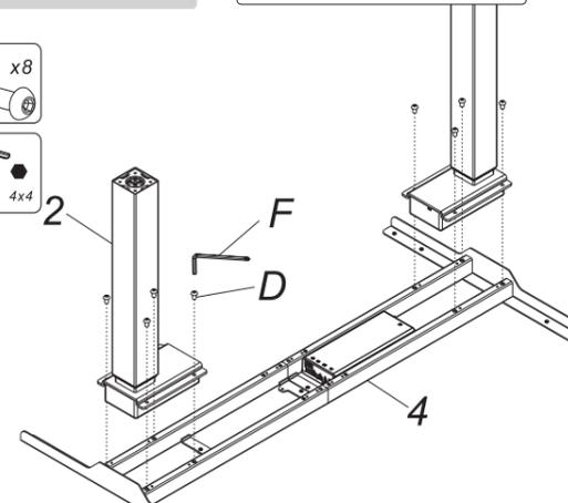
Insert the lifting columns (2) into the ends of the supporting beam(4). Fix the lifting columns using screws(D) with the Allen Key(F).
