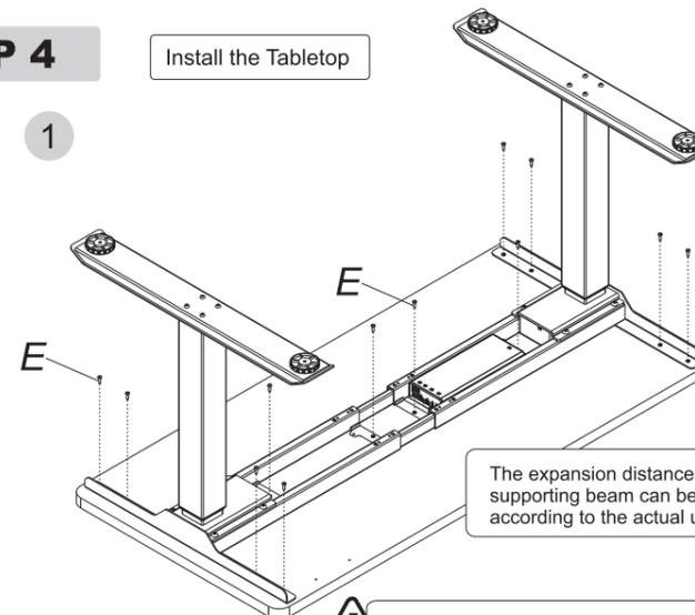
The expansion distance of the supporting beam can be adjusted according to the actual use.
