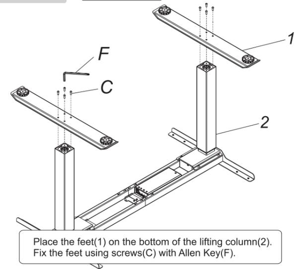
Place the feet(1) on the bottom of the lifting column(2). Fix the feet using screws(C) with Allen Key(F).
